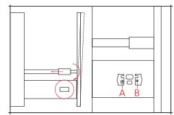
The angle of the drawer front can be adjusted by rotating the drawer bar. The width and height of the drawer can also be adjusted.
