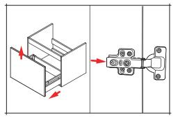
Before mounting the unit, we recommend removing the drawer/doors. To remove the drawer, it should be fully extended and pulled upwards. The entire drawer will release from the guides.
