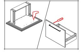
To ensure the paint does not come off the front panel, place the drawer/door (front face down) on a piece of wood. Drill the pilot holes for the handle width selected.
